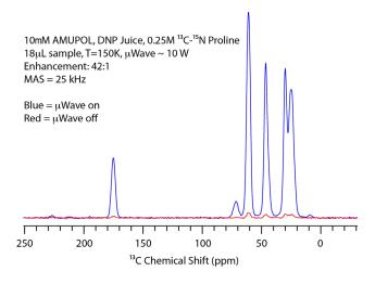
$^{13}C$  CP/MAS DNP enhancement of 42:1 was measured  $^{1,2}$  using a PhoenixNMR 395 GHz/600 MHz DNP HFXY probe fitted with a 2.5 mm spinning module. Sample Temperature = 150 K at MASS = 25 kHz. The sample was prepared using 10 mM AMUPol biradical and "DNP Juice" =  $d_8$ -Glycerol/H<sub>2</sub>O/D<sub>2</sub>O in a 6/3/1 ratio.
