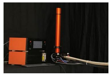
The PhoenixNMR MAS-DNP probe system: a) WB Quad Resonance HFXY probe, b) MAS controller, c) VT cryogenic and sample insert/eject controller, d) Cryogenic counter-flow heat exchanger. Not shown: 50-liter LN2 Dewar. The 50-liter Dewar provides  $^{\sim}36$  hrs of operation at T = 90 K and can be refilled at any time. The included counter-flow heat exchanger is manufactured by Bridge12 Technologies $^{3}$ .
