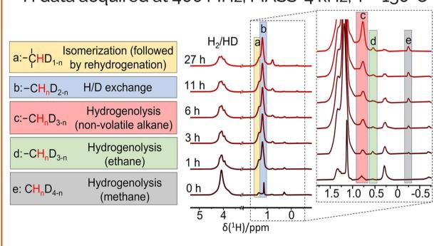
Reactants and catalyst were loaded into a PhoenixNMR HPHT 5mm rotor, pressurized to 300 psi with  $H_2$  gas, then heated to 300°C. At times shown, the rotor was transferred to a standard HX probe and NMR data collected at 150°C.
